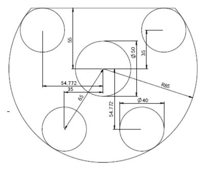
Figure 5. Standard Vision Pattern Dimensions
